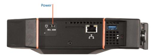
While charging, the LED next to the connector is red. When the battery is fully charged, this LED becomes green.
